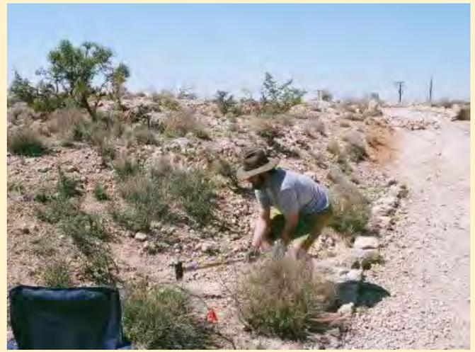
Sometimes geology looks like this: Collecting seismic reflection data in the Odessa Meteor Crater, Ector County, TX. Over a couple of days a railroad tie plate was pummeled with a sledge hammer to produce energy for the survey. It was hit enough times to destroy the plate. Cross section and aerial photo found online.
